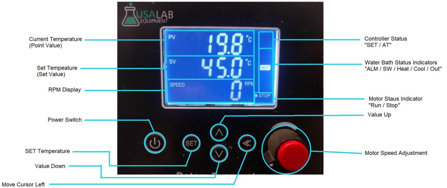
**Temperature:** To set the temperature of the bath. Press the SET button and then use the UP or Down arrows until the Set Value is reached. You can use the left arrow for large changes. Press SET again to finalize the changes.
