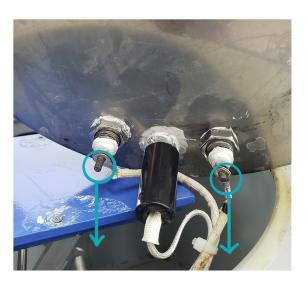
STEP 4: Once the crimped wires are removed, you can then remove the washers and begin to remove the other set of nuts on both sides of the heating element.
