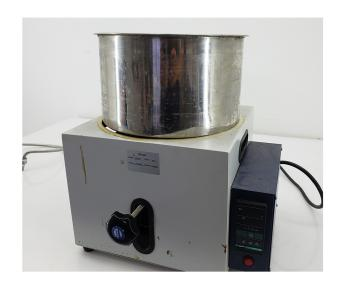
STEP 2: Remove the two screws located at the bottom of the bath reservoir. Once removed, the bath will now be movable from the jack.
