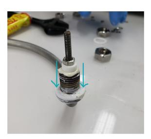
**STEP 8:** Press the heating elements firmly into the bath holes until fully seated.
