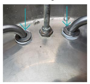
STEP 9: Reconnect nuts, washers and crimped wire in the reverse order from removal. The short crimped wire goes to the right connection, the long crimped wire goes to the left connection.
