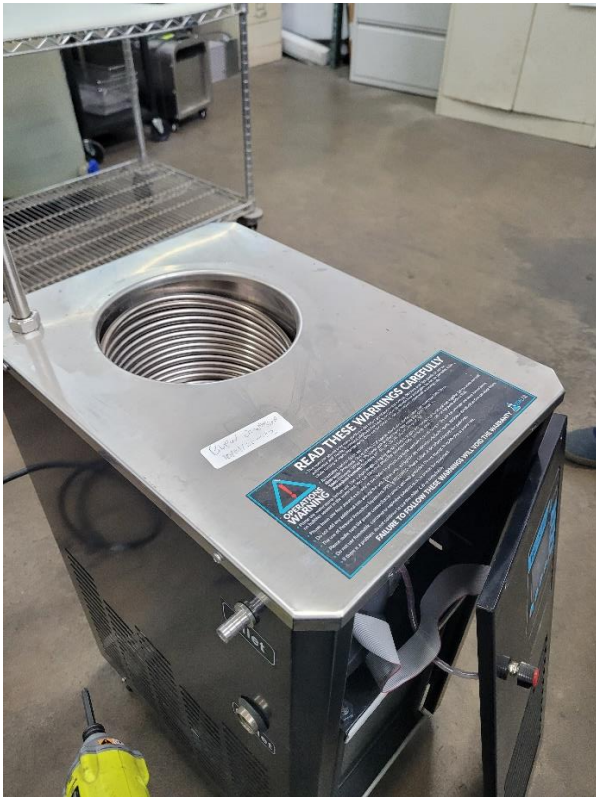
Step 2 | Remove top panel [6 additional screws + 1 large nut]
