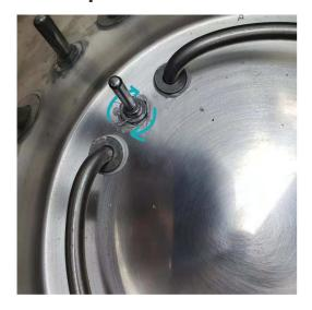
**STEP 8:** Reinstall the probe housing and tighten the set screw.
