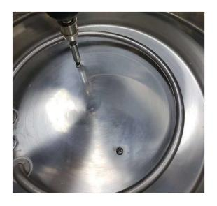
STEP 3: Remove the set screw from the probe housing underneath the bath. You can then unscrew the probe housing from the bath and pull out the probe.
