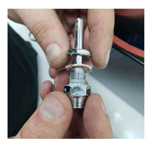
**STEP 5:** Grab the new probe cover and apply silicone around the copper washer as pictured below.
