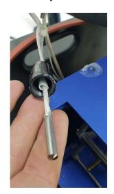
STEP 4: Remove the top probe cover with a 17mm socket. You may need to hold the underside of the probe cover with a wrench to provide leverage. Once unscrewed, you can remove the probe cover.
