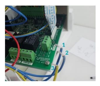
**STEP 2:** Unscrew the probe connector and remove it from the housing.
