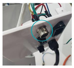
**STEP 4:** Screw all three wires into the PCB connector. (Wiring diagram below)
