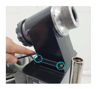
**STEP 2:** Remove the 4 screws for the back plate.
