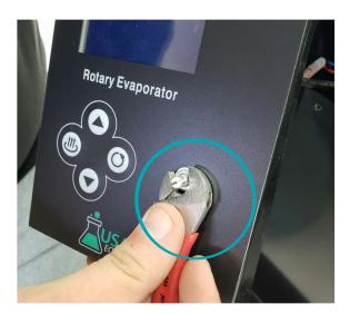
STEP 4: Remove the five nuts holding the display board to the display housing. Once removed you can pull the display board away from the display housing.
