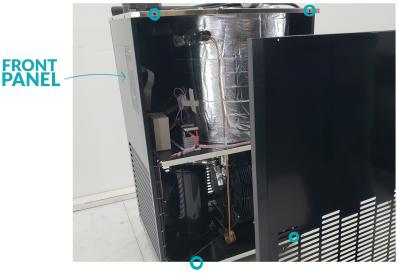
**STEP 2:** Remove the zip tie that is attached to the fan cable.
