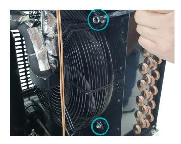
STEP 4: Remove the left side panel. BE CAREFUL. THIS PANEL CAN NOT REMOVE FULLY DUE TO THE INLET AND OUTLET PORTS. ONLY PULL THE REAR OF THE PANEL OUT BEING CAREFUL TO NOT DISTURB THE LINES. You can then remove the other two bolts from the fan housing near the rear.
