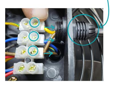
STEP 8: Remove the power cord once the terminal screws are removed. You can install the new fan in reverse order.
